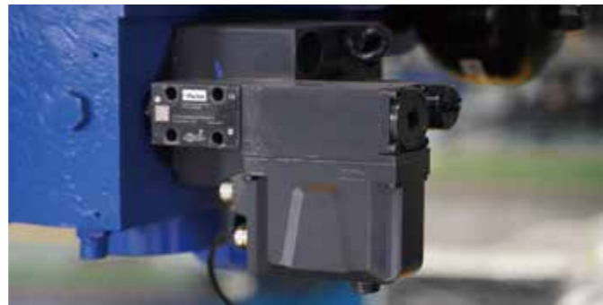
Quick-exit servo valve (dual closed-loop real-time control system)
