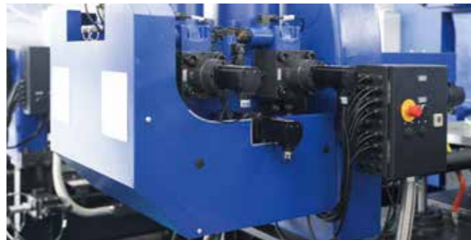
Optional semi-closed-loop injection system: equipped with motorized valve + injection curve for automatic speed/pressure regulation and correction
