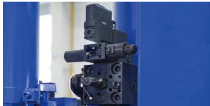
Optional dual closed-loop real-time injection system: quick-inlet + quick-outlet + boost-outlet servo valves enabling closed-loop control of pressure/speed
