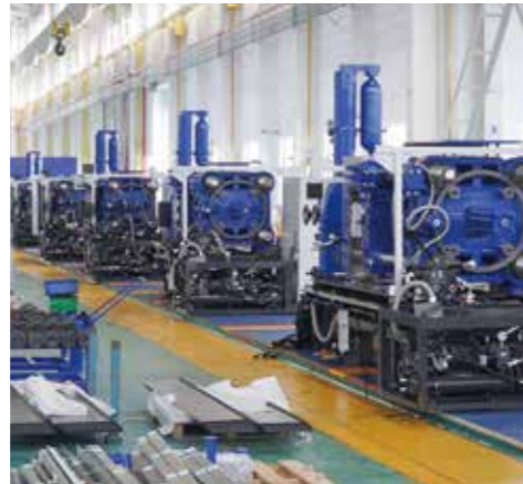
Automated assembly line of die-casting machine
