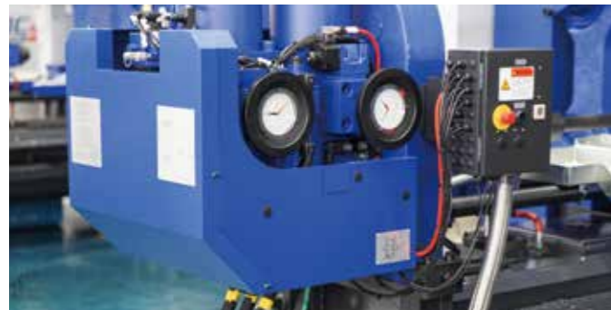
Standard injection system: multi-stage acceleration control adopted, with customized second-stage intensification valve and optimized runner design to achieve exceptional acceleration performance and high stability.
